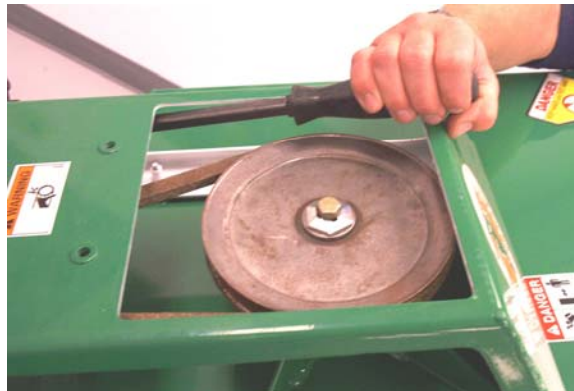
Adjusting Blade Drive Belt Tension
