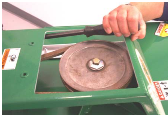
Adjusting Blade Drive Belt Tension
